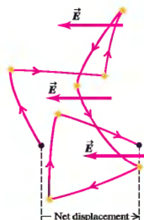
(a) Typical trajectory for an electron in a metallic crystal with an internal \vec{E} field
