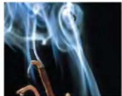
14.21 The flow of smoke rising from these incense sticks is laminar up to a certain point, and then becomes turbulent.
