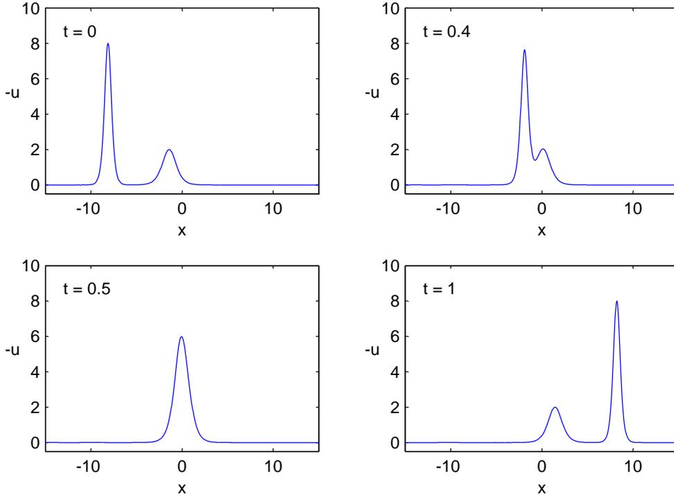
Figure 3.1: Result of simulation of the KdV equation with initial condition given by the two-soliton solution (2.6) with  $t = -0.5$ . Note that  $-u$  is plotted against  $x$ .
