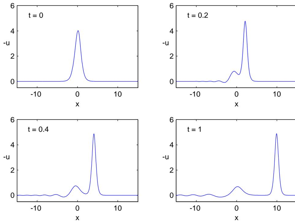
Figure 3.3: Result of simulation of the KdV equation with initial condition  $u(x, 0) = -4/\cosh^2 x$ . Note that  $-u$  is plotted against  $x$ .
