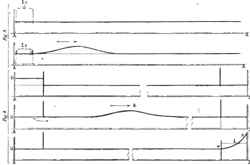
Figure 2.1: Illustration of water tank experiments carried out by Russell. Original image from Ref. [12].
