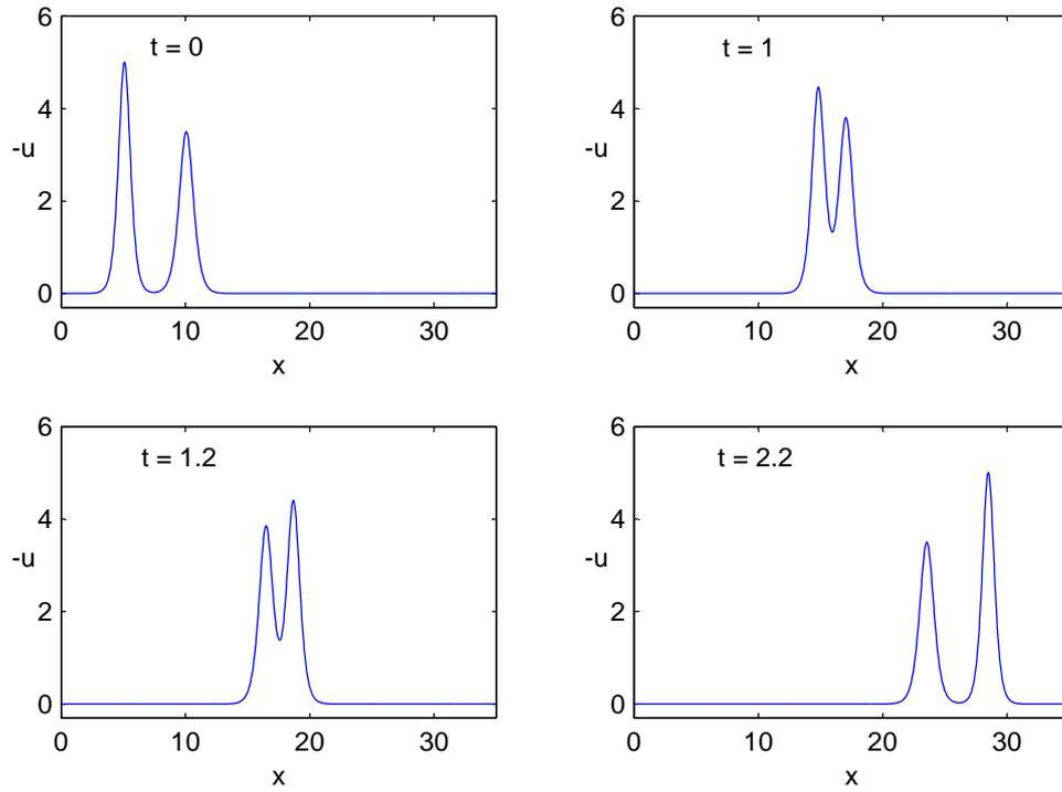
Figure 3.2: Result of simulation of the KdV equation with initial condition given by a superposition of two one-soliton solutions of the form of Eq. (2.5). One soliton has  $c = 10$  and  $x_0 = 5$ , the other has  $c = 7$  and  $x_0 = 10$ . Note that  $-u$  is plotted against  $x$ .
